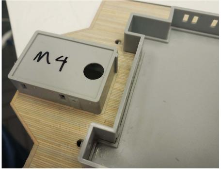
In some places I got the margin planking really perfect. Notice the margin around M4, as well as on the main bulkhead off the upper right corner of M4. Spot on!
