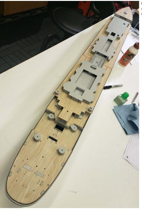
Here is an overview, stern to bow, of the lower 4 decks. These are on sheets 1 and 2, and they are very close to nearing completion. Note the black waterways around the edges of the decks, as well as the leather expansion joints.
